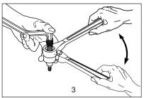
4. Place the ratchet wrench over the hexagonal nut on the tool shank.
