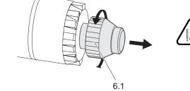
Attention Material damage! If you do not know the stroke setting, unscrew the adjustment screw (6.1) a few turns (ca. 5 mm) for the automatic switch over to the left-handed rotation. This is to ensure that the piston will not hit the back and the riveting tool will not be damaged.
