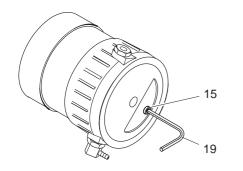
The adjustment to another working stroke follows on the underside of the riveting tool. For this you need the spanner for internal hex key SW4 (19).
