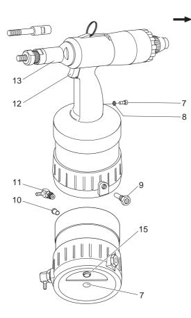
The socket head screw (7) and the O-ring (8) are screwed tightly into the grip. The socket head screw (7) must not be loosened, else the hydraulic oil will leak.
