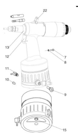
**Note** The socket head screw (7) and the O-ring (8) are screwed tightly into the grip. The socket head screw (7) must not be loosened, else the hydraulic oil will leak.
