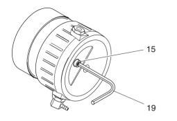
The adjustment to another working stroke follows on the underside of the riveting tool. For this you need the spanner for internal hex key SW4 (19).
