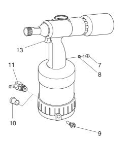
**Note** The socket head screw (7) and the O-ring (8) are screwed tightly into the grip. The socket head screw (7) must not be loosened, else the hydraulic oil will leak.
