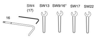
You will require the following tools for all installation, servicing and maintenance work. The tools SW13, SW9/16", SW17, SW22 can be ordered.
