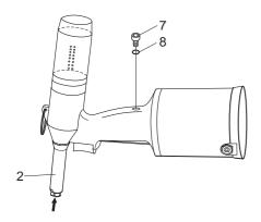
• Bend the riveting tool carefully towards the front at an angle, and fix e.g. inside a vice (like illustrated in the diagram).
