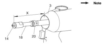
At the time of replacing the jaws, it may be observed that the lock nut (20) at the jaw case body (18) loosens and adjusts itself. In such a case, the gap between X needs to be read-justed (see "Adjusting the jaw case body").
