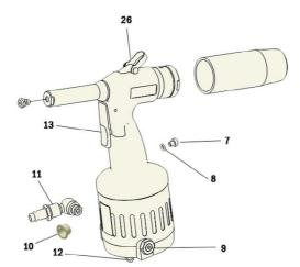
The socket head screw (7) and the O-ring (8) are screwed tightly into the grip. The socket head screw (7) must not be loosened, else the hydraulic oil will leak.
